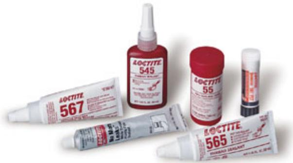
Loctite® liquid thread sealants seal and secure metal pipes and fitting, the space between threaded metal parts, and hardening to prevent leakage. Designed for low and high pressure applications, liquid thread sealants seal instantly for low pressure testing. When fully cured, they seal to the burst strength of most piping systems.
