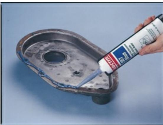
Loctite® silicone gasketing materials include unique products with excellent fluid resistance, formulations for high operating temperatures and UV-curing formulations for cure-in-place production requirements. Silicone gasketing products are best suited for large gap applications and stamped metal assemblies where flange flexing occurs.
