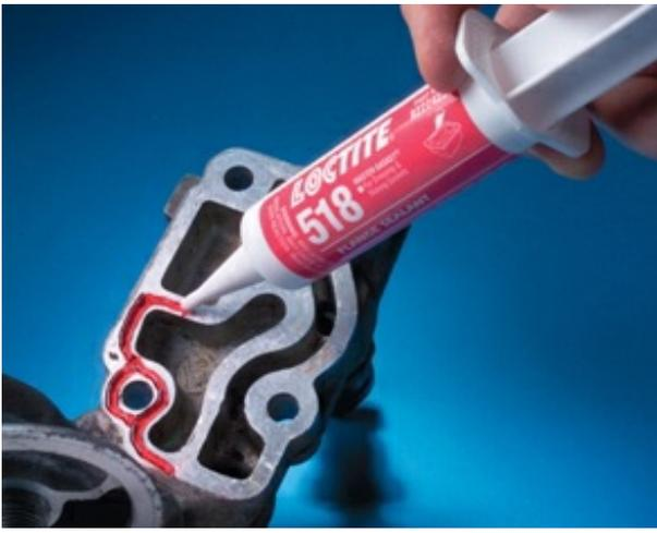
Anaerobic gasketing technology has revolutionized flange sealing in the automotive industry, the assembly of heavy equipment, and the manufacture of various types of fluid power equipment. Loctite® anaerobic gasketing materials remain liquid when exposed to air, but cure when confined between mating flanges. Anaerobic gasketing products are best suited for small gap applications and rigid metal-to-metal assemblies.
