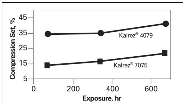
smaller and lighter mechanical seals, which are expected to perform as efficiently as larger mechanical seals. The smaller mechanical seal designs, with reduced spring force retention, put additional demands on elastomeric O-rings with reduced cross sections. The smaller cross section O-rings are more prone to
