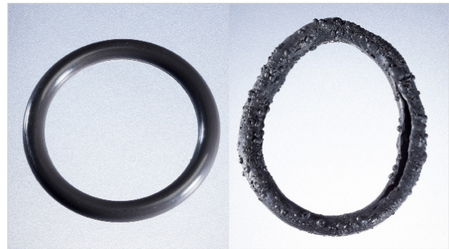
Prior Best-in-Class solution: before/after one week in 600°F steam
